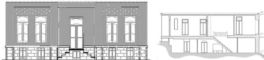
Fig. 9. Elevation and Section of Manafzadeh House
