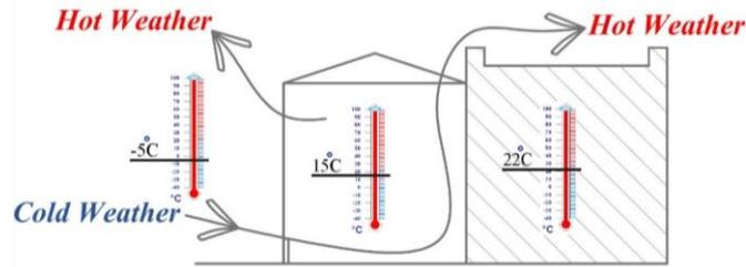
Fig. 67. The diagram shows winter-courtyard as a buffer zone for this type of design
