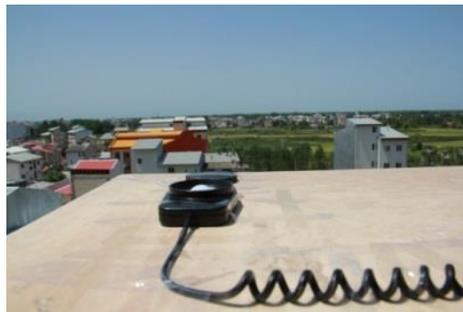
Fig 5: Luxmeter logger (LX-1128SD)
