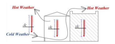
Fig. 67. The diagram shows winter-courtyard as a buffer zone for this type of design
