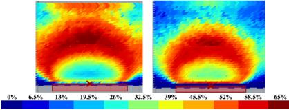
Fig 15: Distribution rate of above 100 lux daylight illuminanceon the working plane during the year. Right: The first optimal window with minimum TEC, Left: The eighth optimal window, (The largest one)
