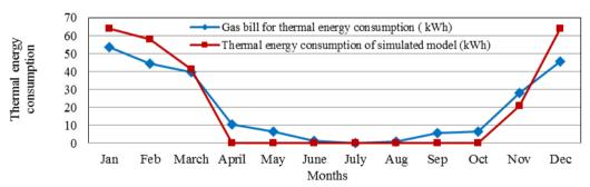
Fig 8: Comparison of monthly thermal energy consumption in 2011 between the gas bills and the simulated data
