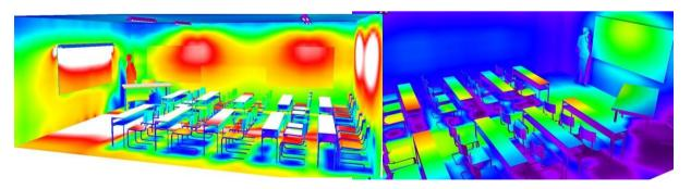
Fig10: Illumination intensity in the classroom. Right: current building. Left: optimal building
