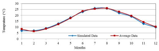
Fig6: Comparison between monthly average temperature data used in the simulation and averages of 5-Year meteorological data
