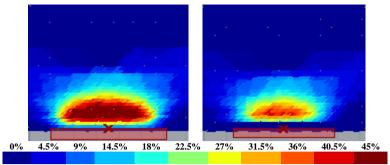
Fig 16: Distribution rate of more than 2000 lux daylight illuminanceon the working plane during the year. Right: The first optimal window with minimum TEC, Left: The eighth optimal window, (The largest one)
