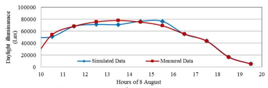
Fig 7: Comparison of daylight illuminance values on 8th August between the measured and the simulated data
