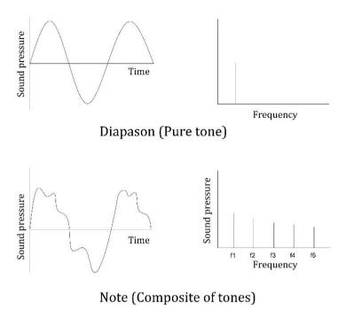
Fig. 4-2: Schematic diagram of pure tone and music note depicts sound pressure changes against time and frequency
