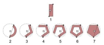
Figure 4. The error resulted from reductionist approach. For all the plans despite different shapes a constant D/2 is calculated as the distance between two exits.
