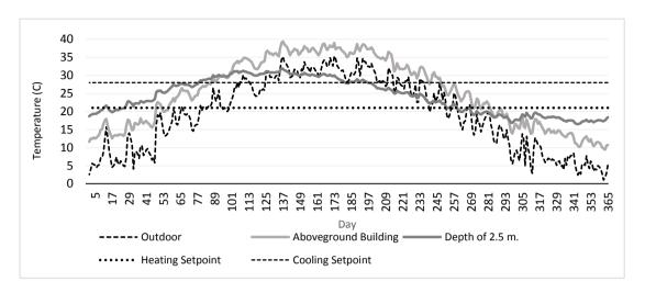
Fig. 5. Comparison of Temperature of Aboveground and Earth-Sheltered
