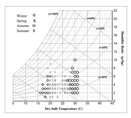
Fig. 7. Earth-Sheltered Building (in depth of 2.5 m) psychometric chart
